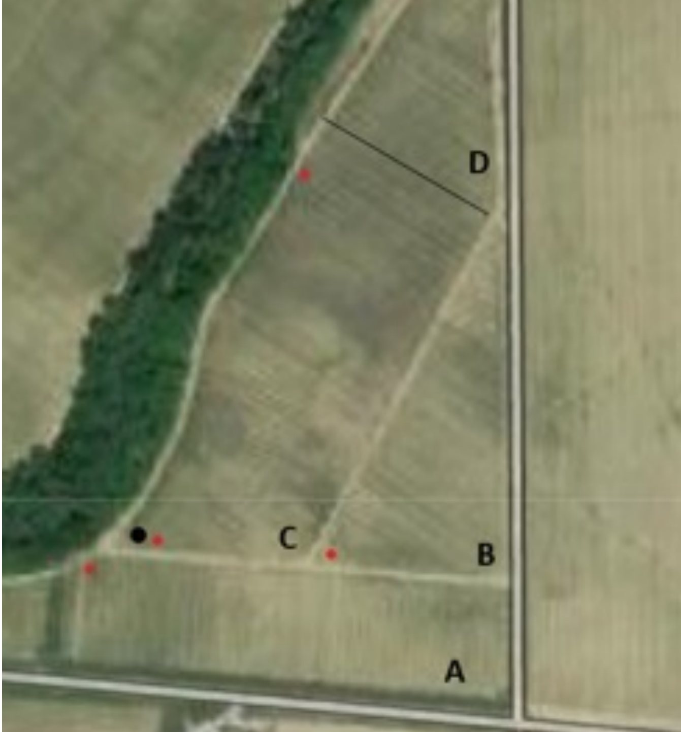
Figure 1. The Cotton Triangle Fields include: the big rectangle (A), the big triangle (B), the trapezoid (C), and the little triangle (D). Red dots indicate risers. The black dot is the well pump.
