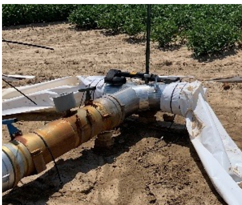
Figure 1 (left). Actuated valve in soybean field. Figure 2 (right). Schematic of automation telemetry communication.
