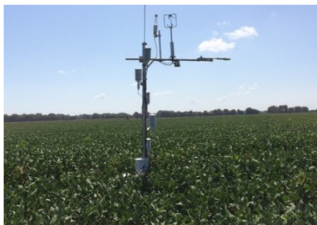
Figure 1. Soybean irrigation experiments equipped with eddy covariance instrumentation for crop water use measurements.
