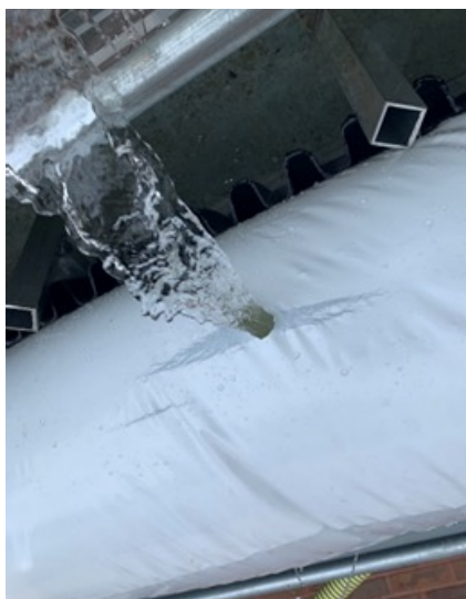
Figure 1. Testing over-pressurized polypipe.
