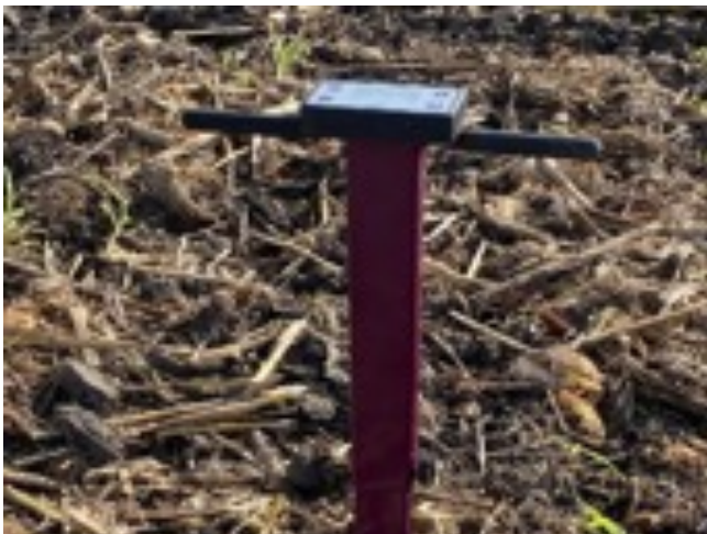
Figure 2a (left) FieldScout TDR 350 being used to collect soil volumetric water content data during the crop growing season; Figure 2b (right) furrow irrigation being applied to an 8 row skip irrigation plot.
