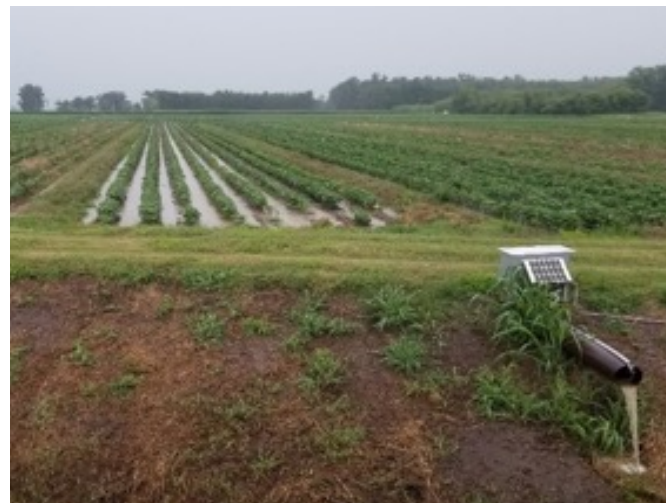
Figure 2. Runoff measurement and sampling equipment.
