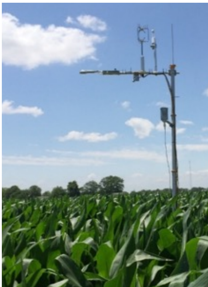
Figure 1. Eddy Covariance sensors installed on towers in a corn field.
