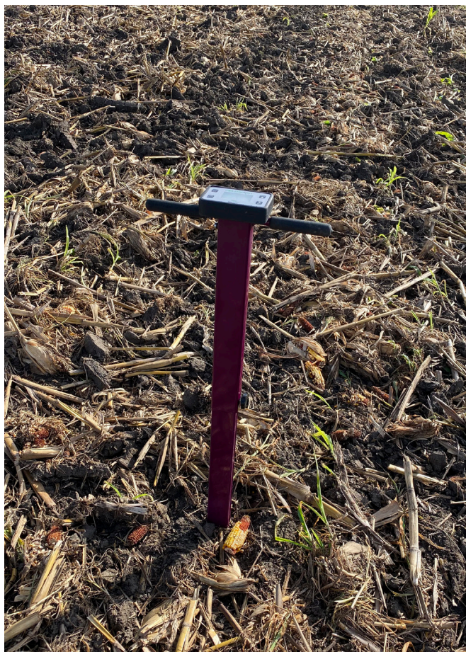
Figure 2. FieldScout TDR 350 was used for collecting soil volumetric water content data during the crop growing season (left) and 8 row skip irrigation treatment showing furrow irrigation water (right).
