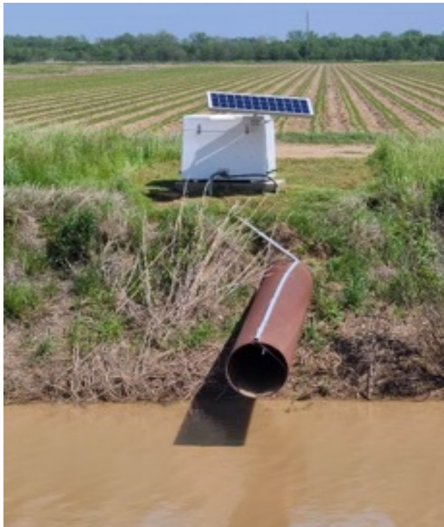
Figure 1a (left) Runoff water sample setup, April 2022; Figure 1b (right) pole with solar panel and storm box for electrical components for the velocity meters under water from November rains which overtopped the tailwater ditch in some places. (Note the flooded fields in the background).
