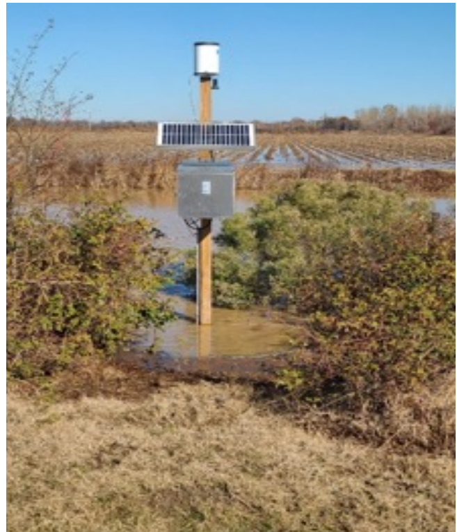
Figure 1a (left) Runoff water sample setup, April 2022; Figure 1b (right) pole with solar panel and storm box for electrical components for the velocity meters under water from November rains which overtopped the tailwater ditch in some places. (Note the flooded fields in the background).
