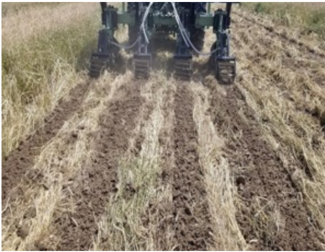
Figure 1. Strip tillage implement in a terminated cover crop.
